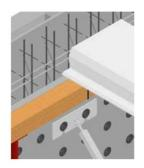
1.2 - The floor element Plastbau® Metal is laid both on the wooden strip and on the internal EPS side (center distance between props 180 cm).
