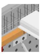
1.1 - The floor element Plastbau® metal is laid only in conjunction with the wooden strip (center distance 120 cm).
