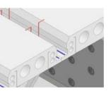
2 - Preparation of the reinforcement rods and iron cages placed all around the perimeter.
