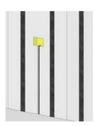
• 3- Use the EPS cutter to make grooves to house the electrical and hydraulic pipe systems.
