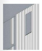
2 - Position the SIP panel into those L-shaped profiles, fix them with some polyurethane glue, and definitively screw the metal profile of the SIP panel to the L-shaped profile.
