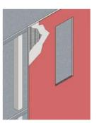
• 4.1- In the case of the external curtain wall, finish the SIP panel with fiberglass mesh and smoothing.
