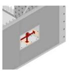
4 - Window compartments are fixed with simple wood planks and props. EPS panels are used to delete thermal bridges. Such a structure is sufficient to resist the concrete casting.
