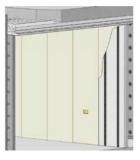
4.2- If used as an internal partition wall, finish with plasterboard sheets screwed directly to the C-shaped zinccoated steel reinforcing profiles.
